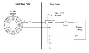
Fig 3 Using a single channel barrier.
