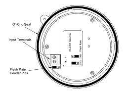
Fig 1 Location of field terminals and controls.
