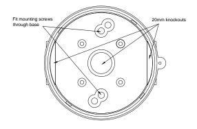
Fig 2 Mounting Beacon Base.
